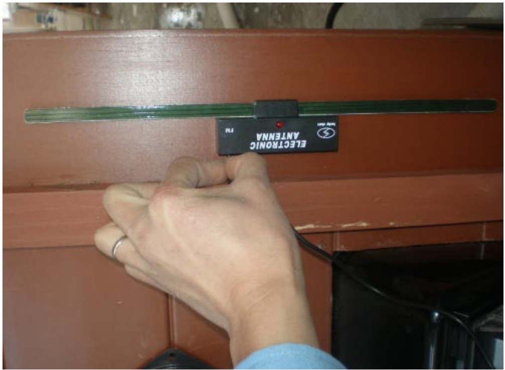
Step 3 Inserts the DVD remote receiver into receptacle on rear of DVD player. As below:
